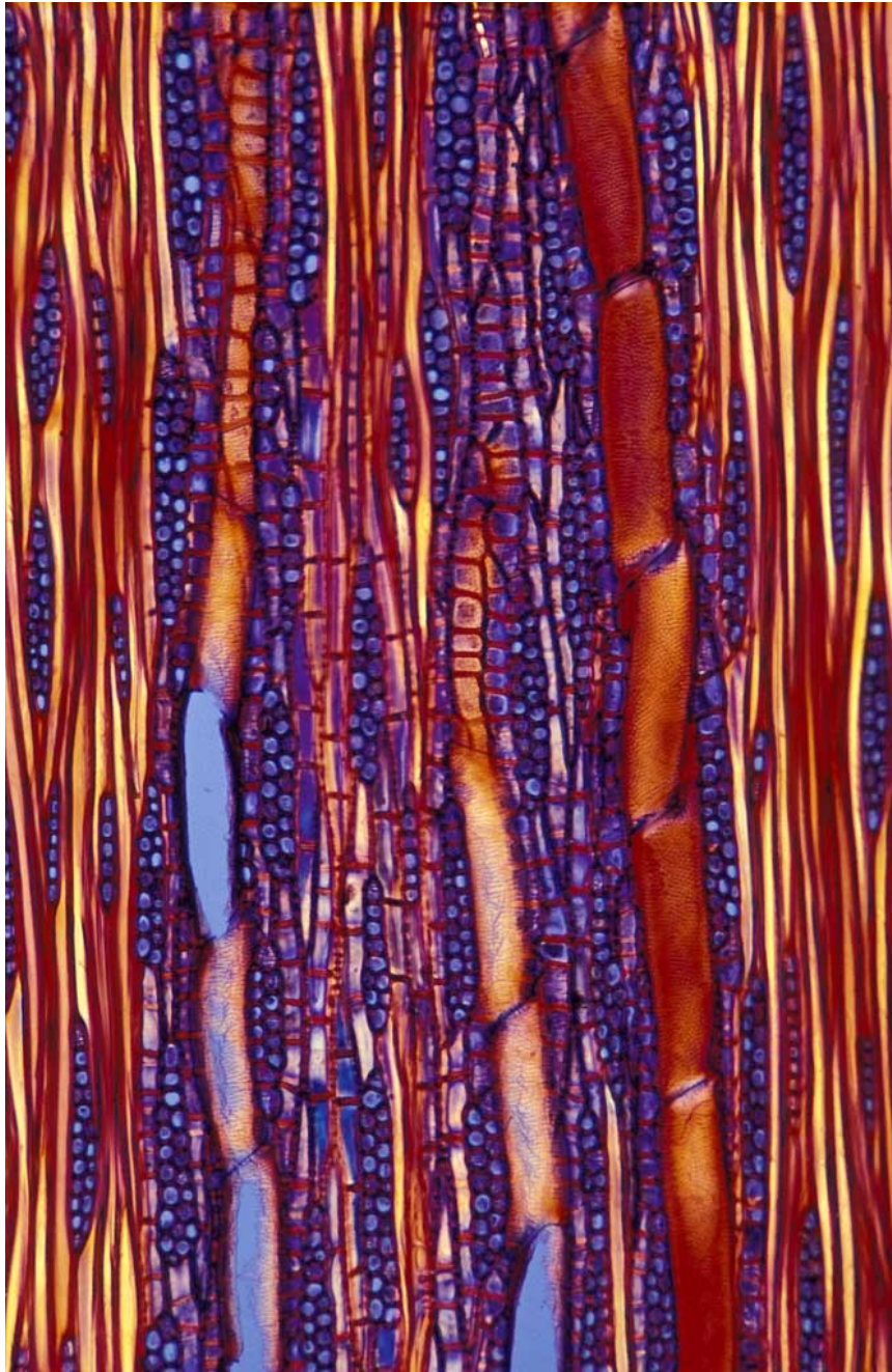
Ash ( Fraxinus americana ) secondary xylem with vessels (LM \times 26 )
